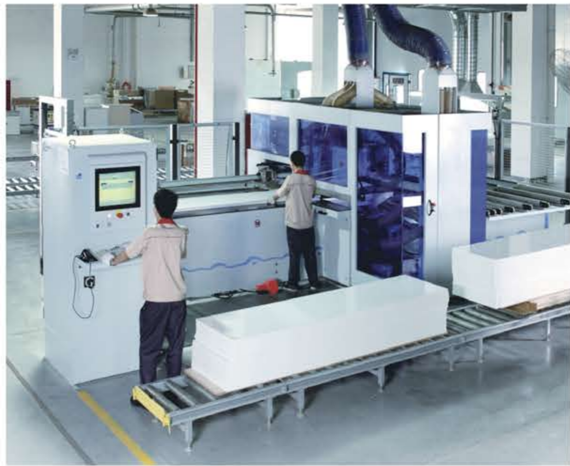
German Homag drilling machine computer controlled
